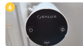
When the LED goes out and TRV head does not make any sounds, adaptation process is finished. Equipment is ready for pairing with thermostat.
