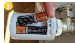
Insert the batteries according to the markings and close the battery cover.
