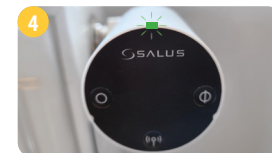
The LED will start blinking green / red informing about the software version.
